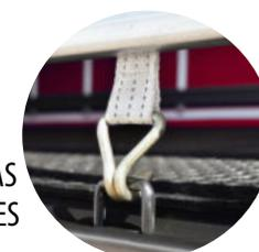
AMARRAÇÃO DE CARGA COM ALÇAS EMBUTIDAS NAS FACES SUPERIORES DOS PERFIS LATERAIS, SEM GERAR INTERFERÊNCIA COM A CARGA, QUE PERMITE UM PROCESSO SIMPLES, SEGURO E RÁPIDO.
