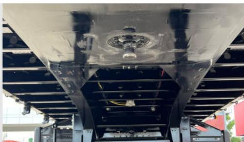
CHASSI COM LONGARINAS VIGAS PERFIL I EM AÇO DE ALTA RESISTÊNCIA MECÂNICA, TRAVESSAS PASSANTES PERFIL C INTERLIGANDO AS LONGARINAS POR SOLDA ROBOTIZADA E CORRIMÃOS PERFIL LATERAL C EM AÇO ASTM A36
