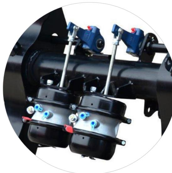
FREIO A AR, COM EBS, LINHAS DE SERVIÇO E EMERGÊNCIA, COM TAMBOR 16 1/2" x 8" E CÂMARA DE FREIO 30 POL<sup>2</sup> COM *SPRING BRAKE* | RESOLUÇÃO 915|22 CONTRAN
